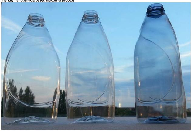
PET flasks with 0, 10 and 250 ppm (from left to right) of new plasmonic nano-ceramic re-heater
